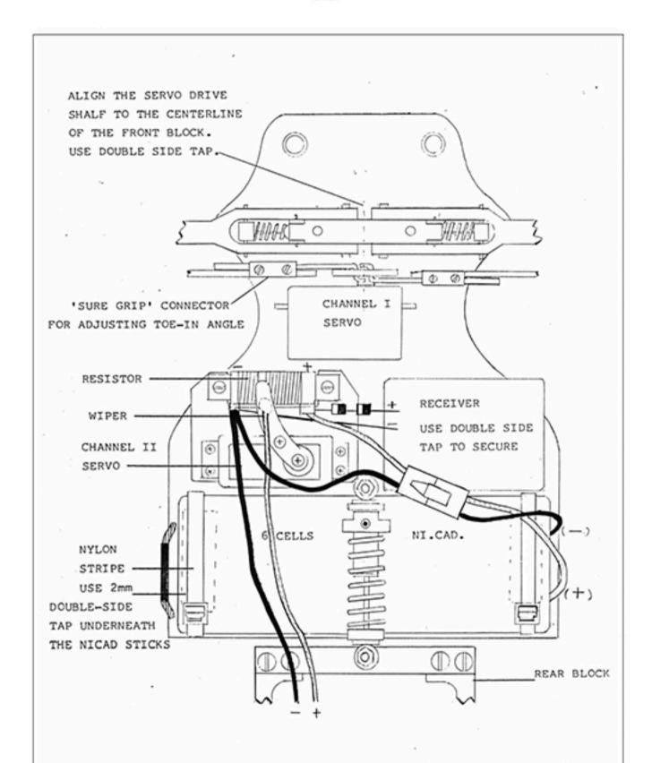
POSITIONING OF R/C SET AND NI-CAD. BATTERY
