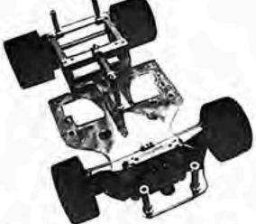
Adjustable front swing arm suspension system can be adapted to other 1/12 racing cars to improve handling.
