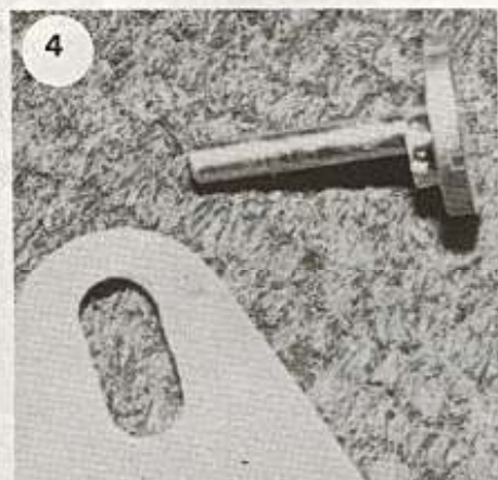
1. Adjustable motor mount, two gear ratios supplied in kit. 2. Single spring loaded servo saver, fits Futaba servos or Powermax Skyranger type shown here. 3. Neat moulded plastic battery retainer lock with cyanocrylate to prevent rotation. 4. Cam and slot tweak adjustment system, very positive in operation. 5. Acoms receiver fits neatly under the shaker plate in front of the battery pack.
